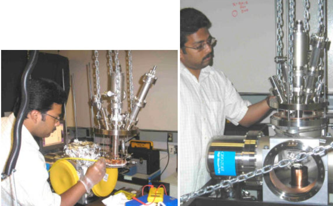
Fig. 3 Graduate student Anoop George is (left) cleaning the particle detector grid with nitrogen gas and (right) lowering the detector-electron gun assembly into the UHV vacuum chamber.
