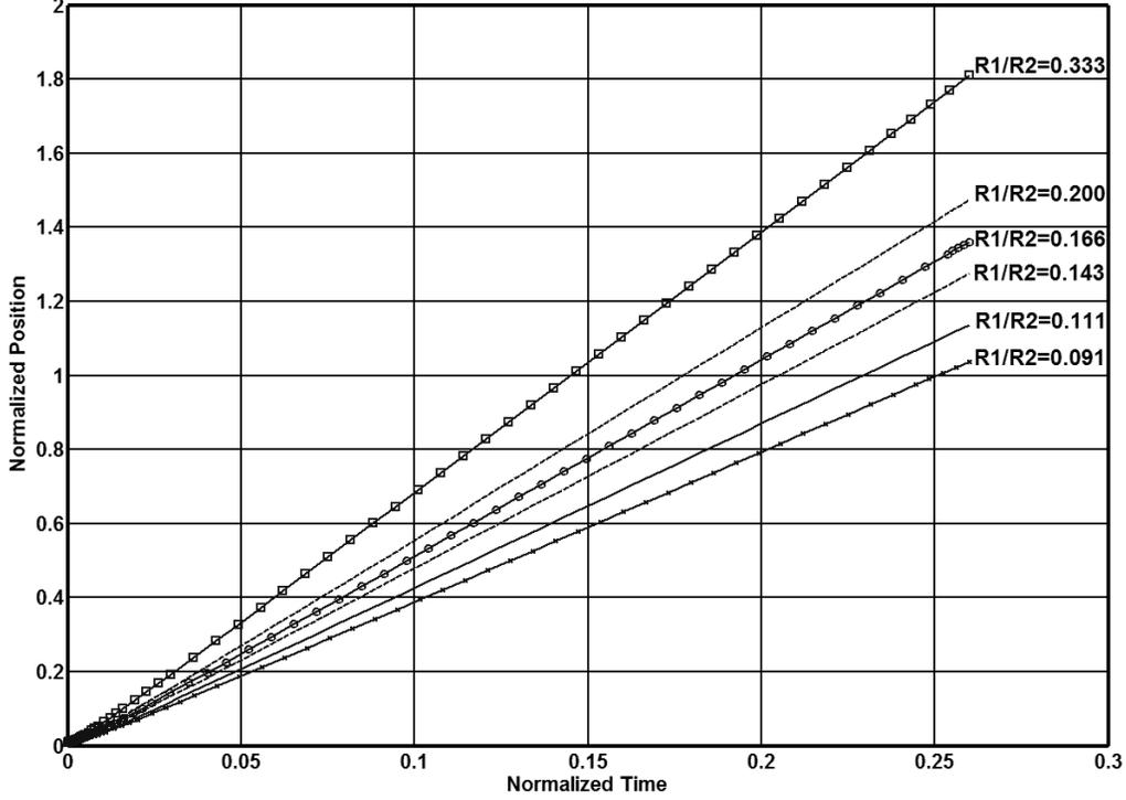
Fig. 1. Displays the normalized radial position of the particle  $\tilde{r}$  with respect to the normalized time  $\tilde{t}$  when the initial motion along the z-axis is zero for various  $\tilde{R}_1$  when  $\tilde{E}_0 = 0.001$ .
