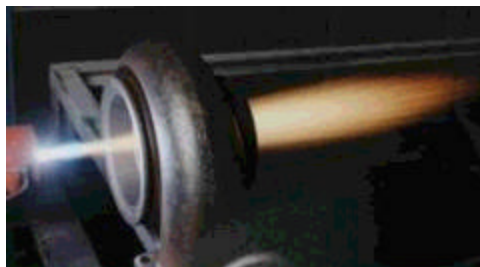
Plasma spraying of high temperature resistance surface coatings for a diesel engine turbocharger housing
